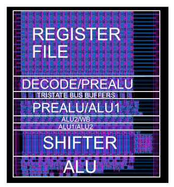
Figure 6. The Scalar Datapath Layout
